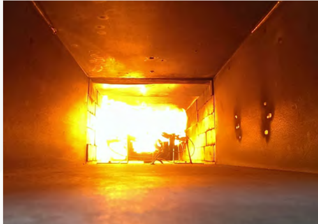
Steiner Tunnel Testing for flame and smoke development
